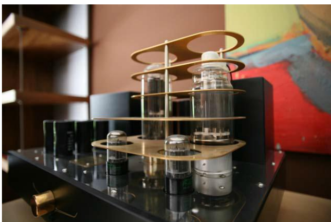
Audio Aero Prestige monoblock power amplifiers, single ended, 40watt@8/40hm pure class A. Price: 8500€
